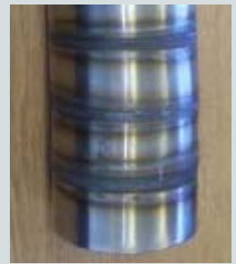
TIG Welded pipe with clear to see thermal oxides present
