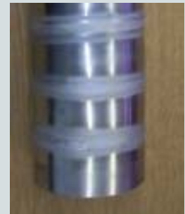
Chemical pickling leaves a uniform matt surface, free of any ferritic contaminants.
