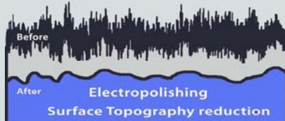
Electropolishing dramatically reduces micro roughness by dissolving metal ions faster at the exposed peaks, leading to lower Ra values, although most important is the smoother surface topography.
