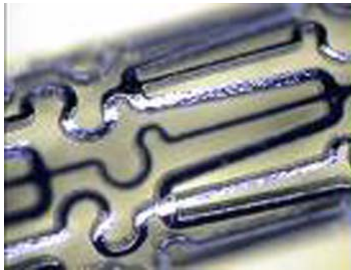
Fig 6 - 7 Shows Cardiovascular Stent after Electropolishing with rounded edge profile
